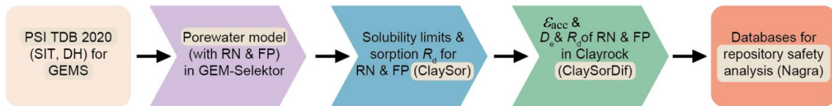
Figure 3: Consistent toolchain of geochemical data and models
